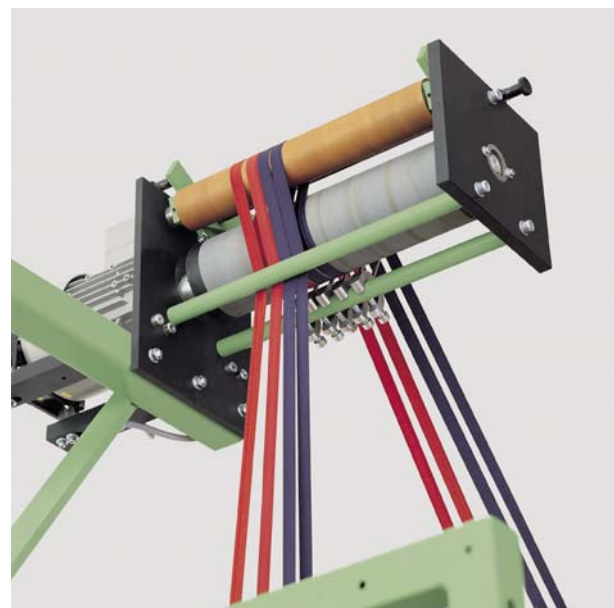
Torque-controlled transport roller for elastic narrow fabrics or very soft windings
