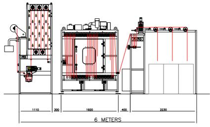
MFR 10C (standard configuration for pigment dyeing /finishing using a 10 cylinder stack)
