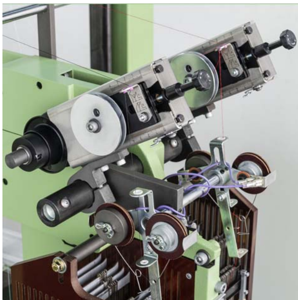
Weft feed with option "Wire spring compensation"
