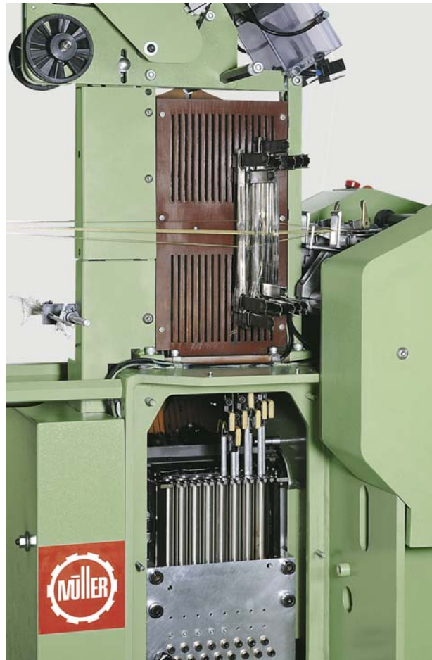
Patented shedding motion with air-suspended heald frame motion
