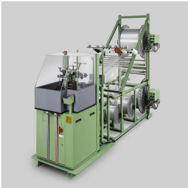
NG3S with sound absorbing enclosure
