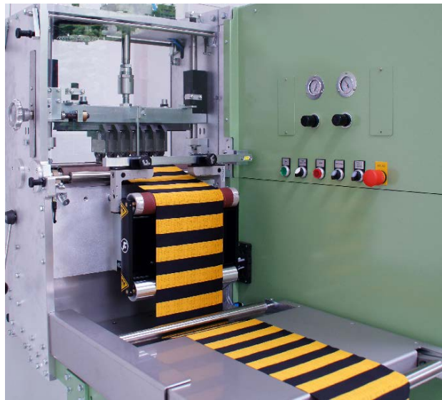
Supply of label ribbon from roll
