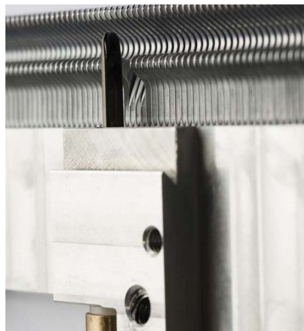
Weft channel with relay nozzles
