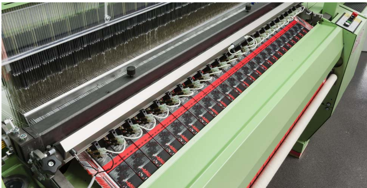
1,200mm working width and TC2 cutting system
